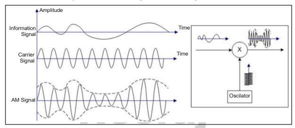
We do amplitude modulation of a signal wave by superimposing it with a carrier generated signal and this causes a change in its amplitude. It is this modified signal and is sent via a transmission:
