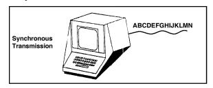
Synchronous transmission means blocking a group of characters in way records are blocked on magnetic tape.
